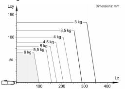
The KR 6 R900 EX is designed for a rated payload of 3 kg in order to optimize the dynamic performance of the robot. With reduced load center distances, higher loads up to the maximum payload may be used. The specific load case must be verified using KUKA.Load. For further consultation, please contact KUKA Support.
