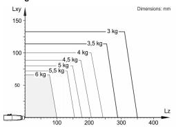
The KR 6 R700 WP is designed for a rated payload of 3 kg in order to optimize the dynamic performance of the robot. With reduced load center distances, higher loads up to the maximum payload may be used. The specific load case must be verified using KUKA.Load. For further consultation, please contact KUKA Support.
