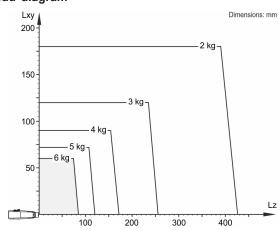
The KR 6 R700 HM-SC is designed for a rated payload of 3 kg in order to optimize the dynamic performance of the robot. With reduced load center distances, higher loads up to the maximum payload may be used. The specific load case must be verified using KUKA.Load. For further consultation, please contact KUKA Support.
