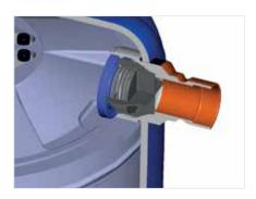
X Non-Return Valve (XNRV) placed inside the discharge connector reduces refrigerant migration from high pressure to low pressure side after the compressor shutdown, improving compressor reliability with no additional costs on assembly for the OEM or installer.
